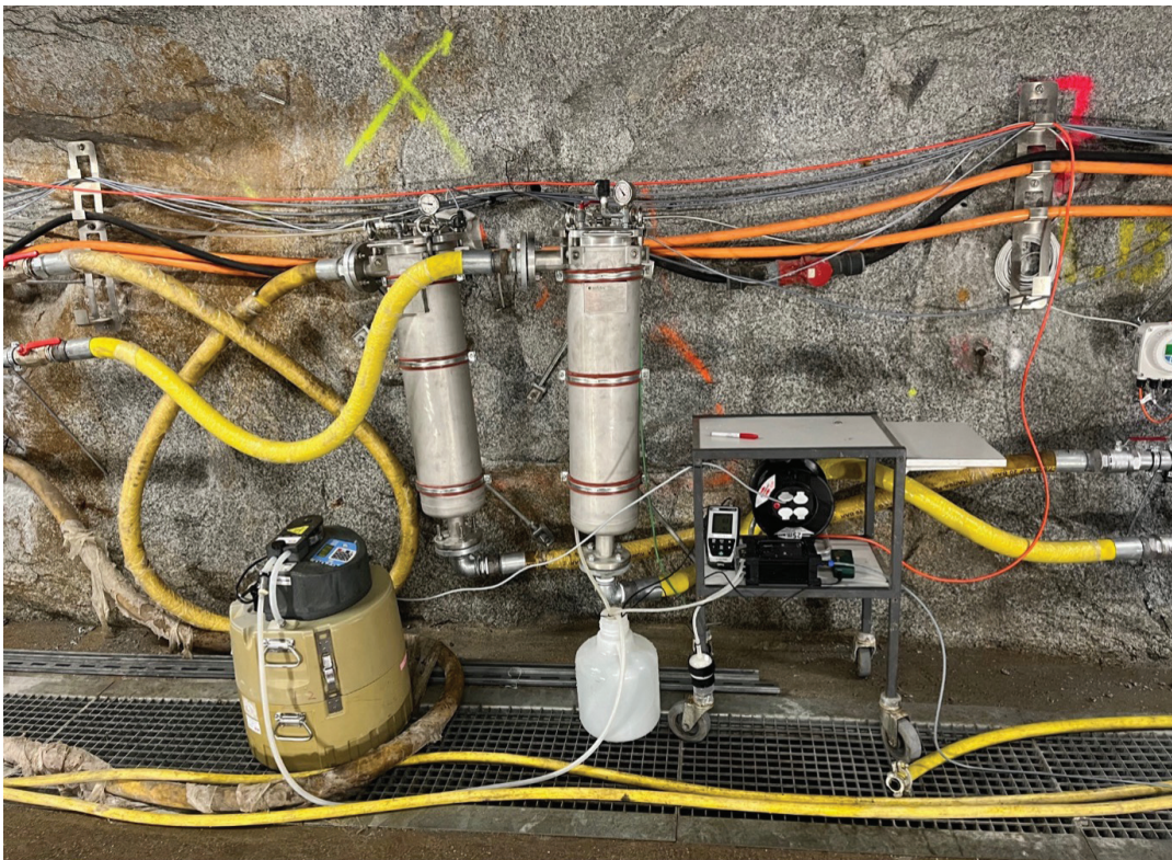
Biogeochemical monitoring setup at the injection tank during the hydraulic stimulation
