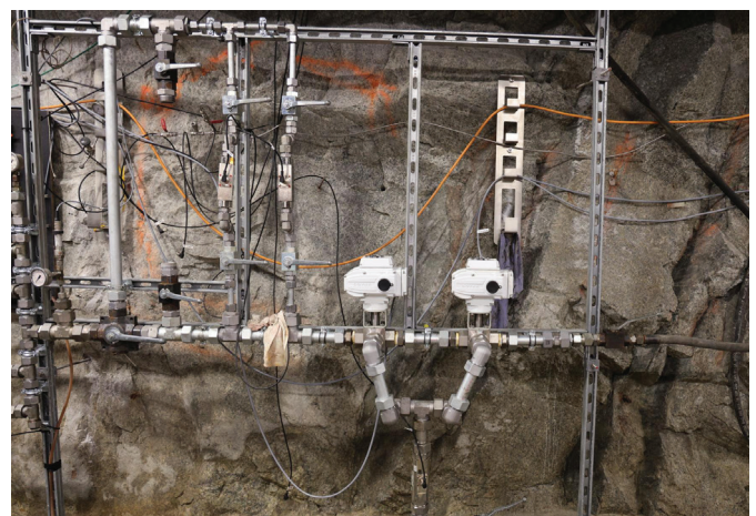
The flowboard including the remotely controlled motors
